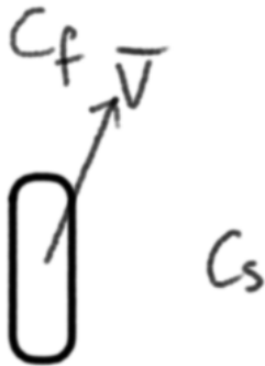
C_f - friction coefficient when wheel moves forward/backward C_z - friction coefficient when wheel moves sideways V - velocity In this case coefficient will be closer to C_f
